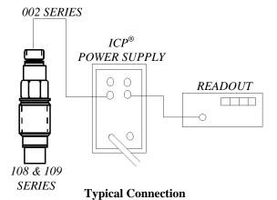
The figure above shows the 108 & 109 Series connected to a PCB Model 484B06 power unit. The 484B06 is a power unit that can be AC or DC-coupled.
